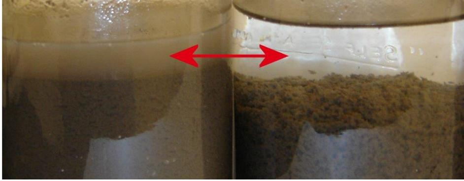
**Figure 8. Settling improvement from Coagulant addition**
