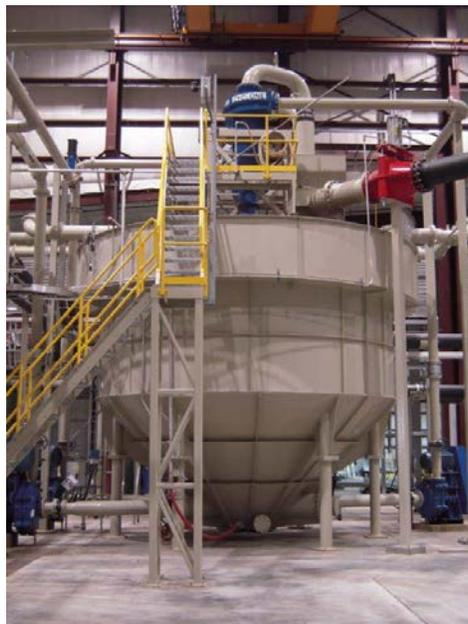
**Figure 1. Thickener tank**
