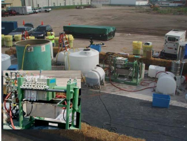
**Figure 5. Plate and frame membrane filter press simulator for onsite pilot testing**
