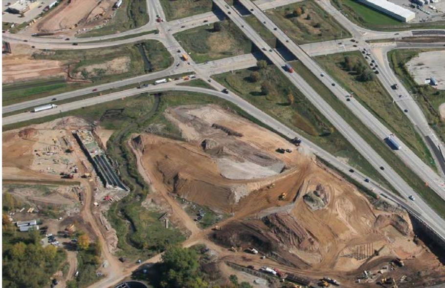
**Figure 7. Aerial photo of US Highway 41/State Highway 29 Interchange showing WisDOT construction using approved sand from Lower Fox River project**
