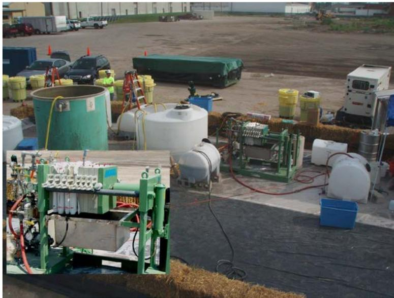
**Figure 1. Plate and frame membrane filter press simulator for onsite pilot testing**
