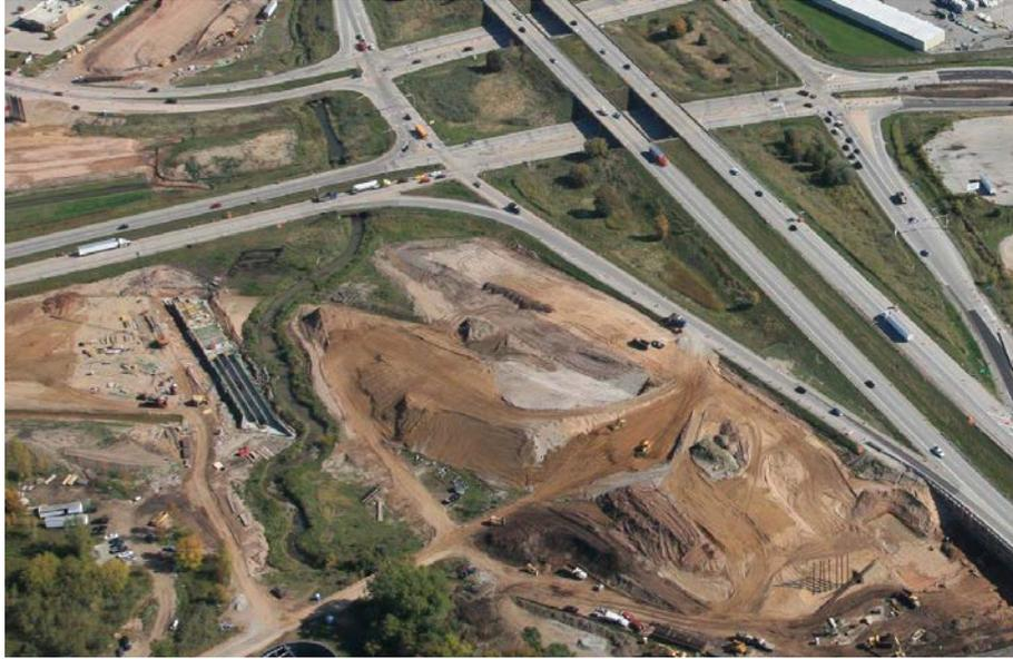
**Figure 4. Aerial photo of US Highway 41/State Highway 29 Interchange showing WisDOT construction using approved sand from Lower Fox River project**
