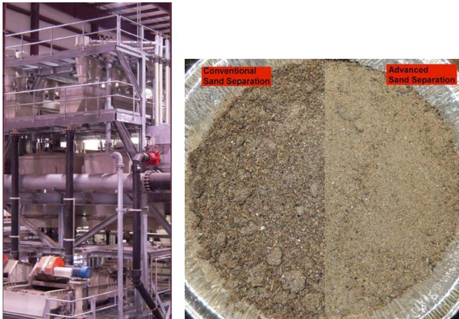
**Figure 2. Advanced sand separation unit and typical resulting product from additional processing step**
